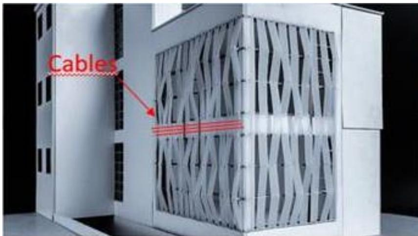
Figure 8 – Schematics of the position of cables of the Booster textile demonstrator.
