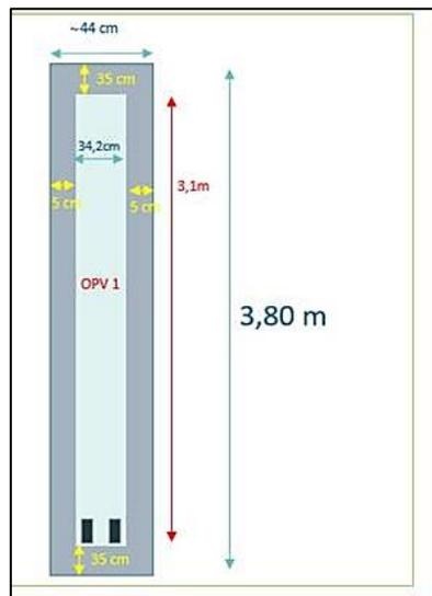
Figure 7 – Schematic top view of the characteristics and sizes of the Booster textile module.
