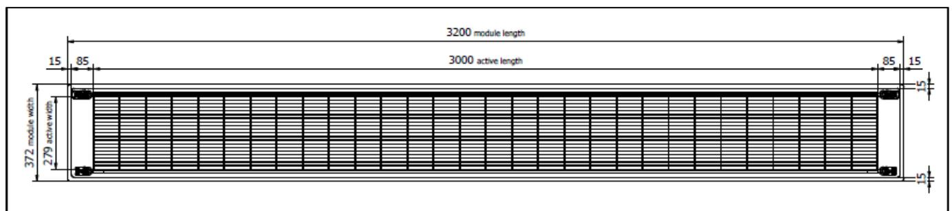
Figure 3 – Schematic top view of the characteristics and sizes of the BOOSTER ready to stick module.
