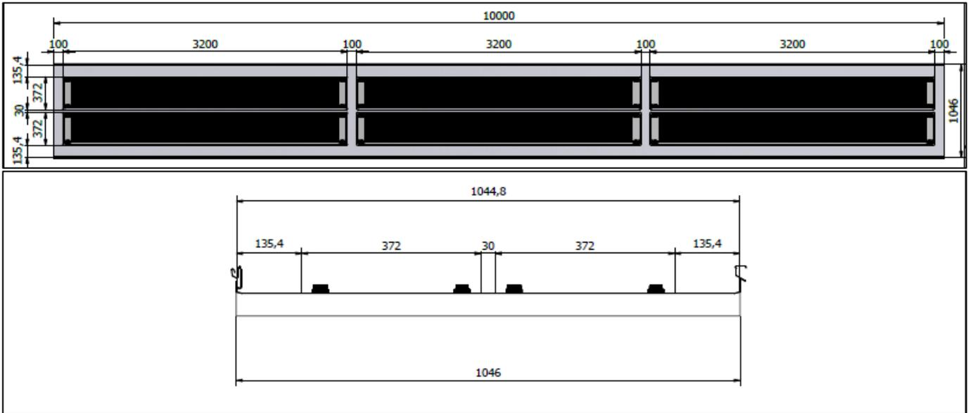
Figure 4 – Top – Schematic top view of one canopy steel module and six Booster ready to stick products attached to it with sizes. Bottom – Sketch of the above schematics viewed in section.
